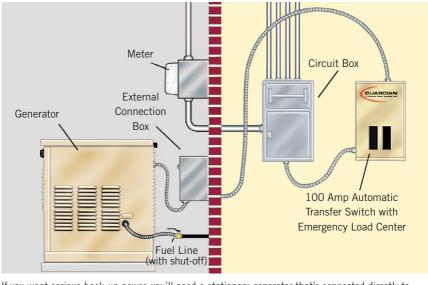
If you want serious back-up power, you'll need a stationary generator that's connected directly to your home electrical system. This setup requires a transfer switch to disconnect from the grid.
